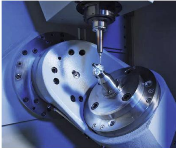
With its new, highly dynamic milling machine, Chiron produces a complete compressor wheel in two minutes
