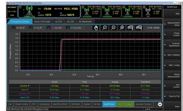
1.6Gbps data throughput with LTE-A 4CC CA with 4x4 DL MIMO from simulated UE
