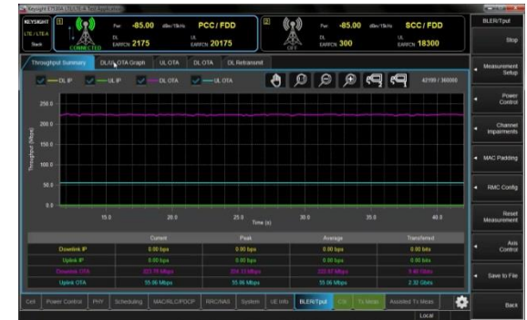
LTE FDD 4x4 MIMO+ TM9 1CC + 64QAM DL ~224.8Mbps (theoretical)
