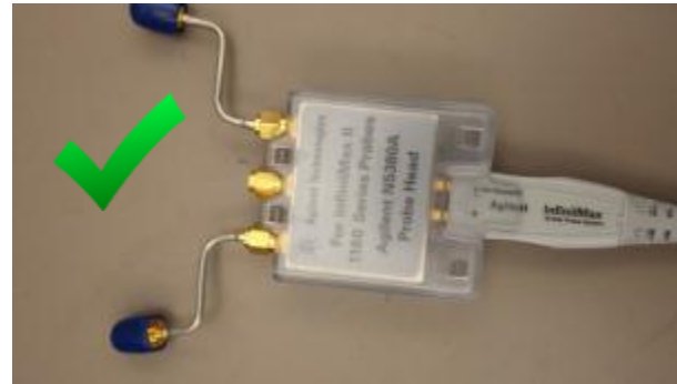
Housing with built-in strain relief (for N5380B SMA head)
