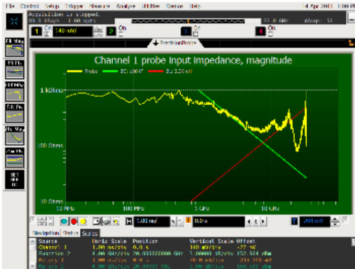
Figures show a solder in probe characterized by PrecisionProbe and a VNA. Notice how closely the characterization matches both systems
