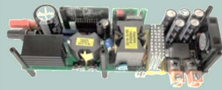
600W LLC Reference Design using XMC4200 Achieves TITANIUM efficiency standard
