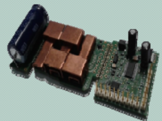
Power Tool KIT using XMC1302 1kW/20VDC BLDC Motor Control
