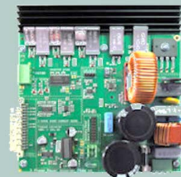
750W power inverter with PFC (115VAC to 230VAC) nominal 3A motor current
