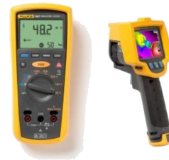
Motor Insulation and core temperatures with Fluke-1507 & Thermal Imagers
