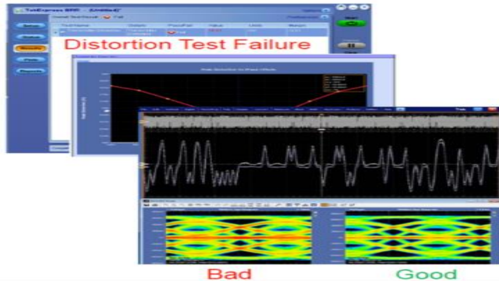
Timing error using DPOJET eye diagram
