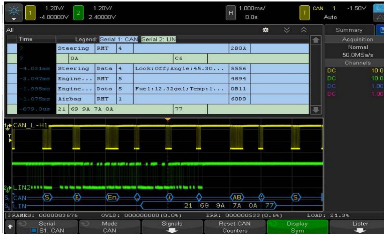
Dual serial bus CAN and LIN decode
