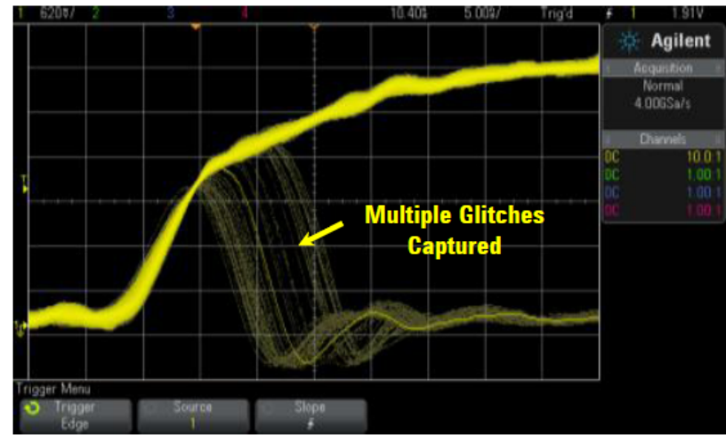
Ex #2: Update Rate = 1,000,000 waveforms/sec
