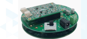
System board stack, bottom side up to show A 2 B interface. 8 microphones on bottom board in above stack
