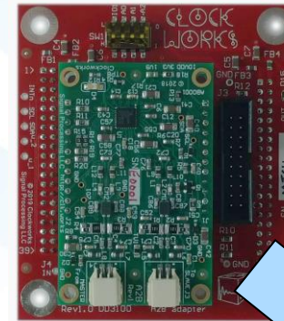
Adapter board with A 2 B module
