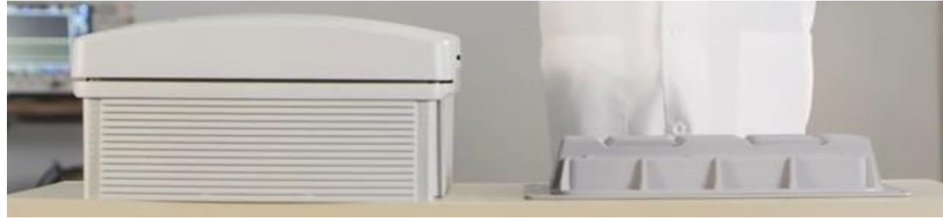
IGBT based 10kW Solar Inverter Forced air cooling, must be de-rated over 45C ambient
