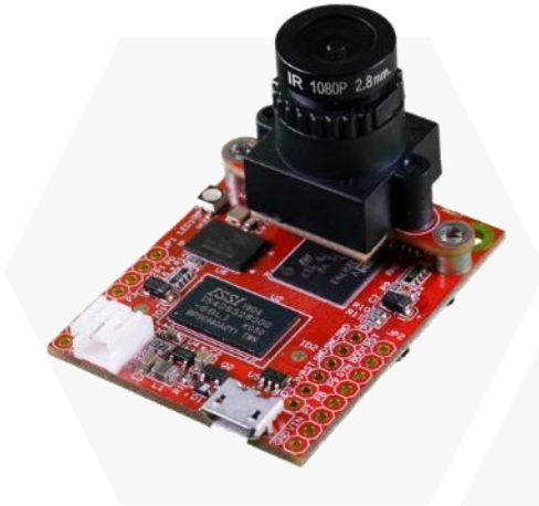
OpenMV CAM Running MicroPython over STM32
