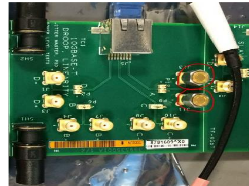
Point to Point test config (100ohm)
