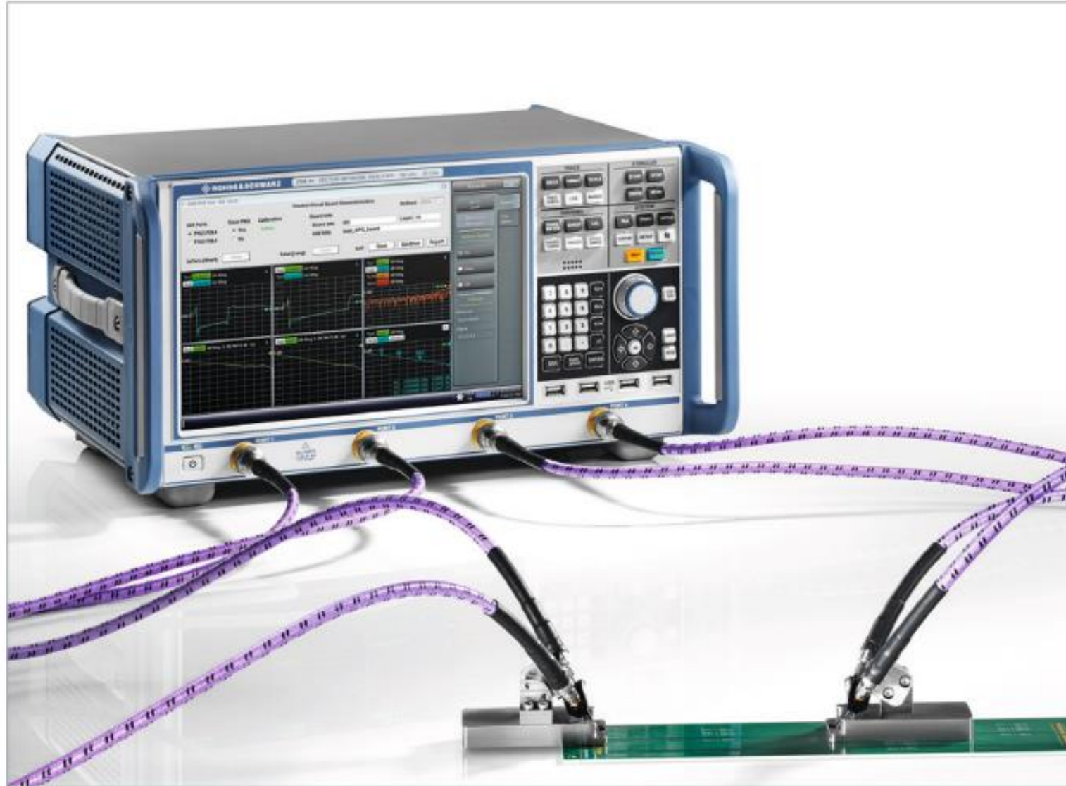
Verification of high-speed differential signal lines.
