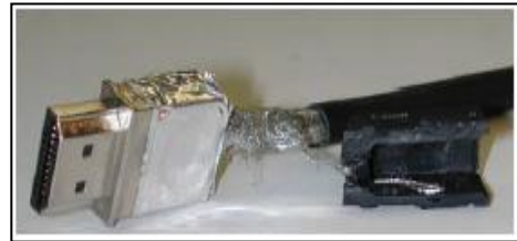
Fig 2. Poorly-shielded HDMI cable with only a few strands of braided shield contacting the metal tape on the plug
