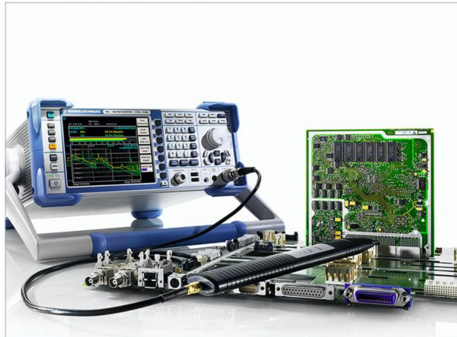
EMI debugging using testreceiver.
