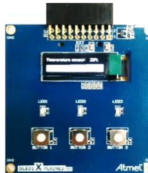
Atmel OLED1-XPRO extension display board. Atmel OLEDIO1 Xplained Pro 128 x 32 Pixels Controlled by 4-wire SPI interface Three LEDs, Three Buttons
