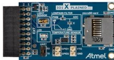
Atmel ATIO1-XPRO Sensor extension board. Atmel IO1 Xplained Pro ADC: Light Sensor and PWM signal filtered into ADC TWI: Temperature sensor w/ EEPROM SPI: microSD card holder + microSD card
