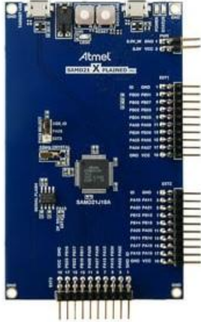
Atmel SMART : SAMD21-XPRO Evaluation kit. Atmel SAMD21 Xplained Pro SAMD21J18A microcontroller 8 Mbit Serial Flash 32.768kHz crystal Embedded Debugger
